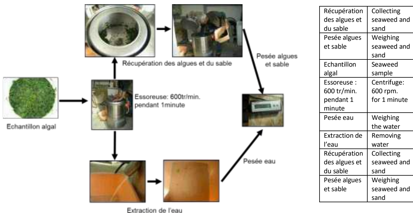
Figure 8: Description of the procedure to directly assess extracellular water content in harvested seaweed
