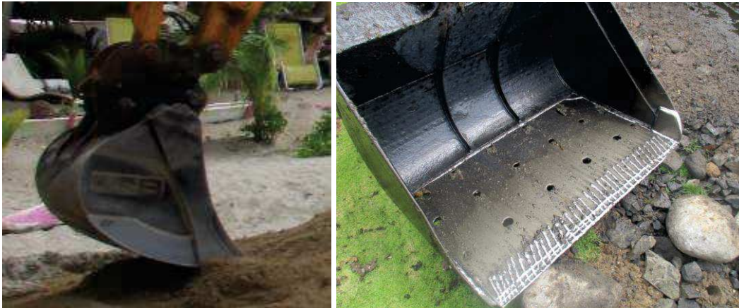
Figure 72: Digging bucket (left) and riddle bucket (right)
