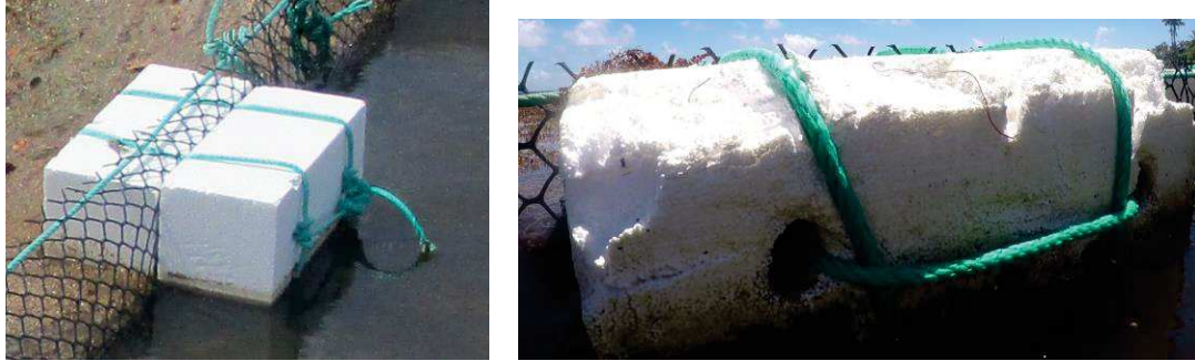
Figure 36: Comparison between the state of floats in June 2018 (left) and September 2018 (right)
